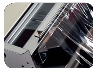
1. Profilo teflonato Teflon-coated section
