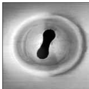
The nozzle geometry of the wide angle nozzle FAN was calculated in numerous simulations.
